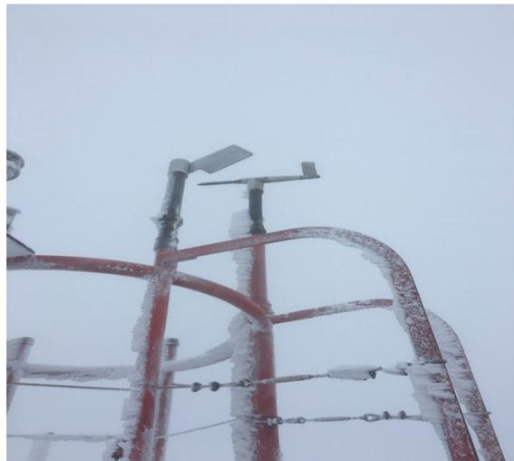
Workers at the Mount Washington Observatory installed the new weather vane created by Andy Shaw's Advanced Manufacturing class. Initial reports from atop the rockpile indicate "that it is easier to de-ice than the old vane. Most likely due to the smooth surfaces compared to the nicked and scarred old one. It also seems to be more sensitive to direction changes, another plus. Our Meteorologists will be conducting longer term studies on this as this will be important to our dataset."
